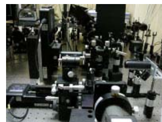
Optical table showing the collinear phase-lock holographic memory recording system
