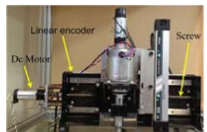
Fig.1: A novel non-linear sliding surface controller for ball-screw feed-drive systems was developed by researchers from the Toyohashi University of Technology. Servo-drive systems are widely used in industry, in particular for power efficiency applications.
