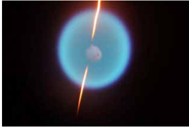
A round flame in a low air pressure environment
