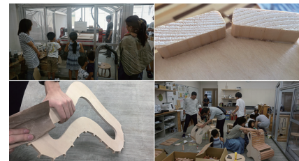
Fig.2 Cutting by CNC router (upper left), detail of fitting part (upper right), manual filling work (lower left), picture of the workshop (lower right)
