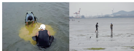
Fig.2 Survey of sediment transport and morphometry of tidal flat Setting up color sand (left), morphometry of tideland (right)
