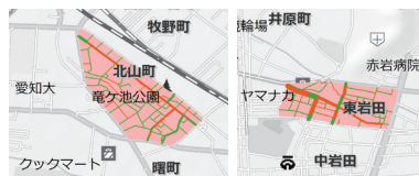
Fig.2 Example of grasping the state of rat-run traffic using GRATT within a "Zone 30": 30km/h limit zone (Line width: amount of rat-road traffic, Green line: average speed less than 30 km/h, Red line: average speed 30 km/h or more)
