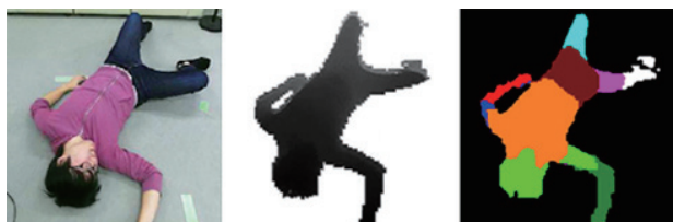
Fig.1 Example of pose estimation using depth data: Left: Experiment scene (this image is not used for estimation), Center: Depth data corresponding to the extracted person region, Right: Estimation result (the colors correspond to each part of the body)
