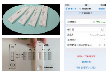
Fig.2 Immuochromatography kit for a detection of residual pesticide in agricultural products.
