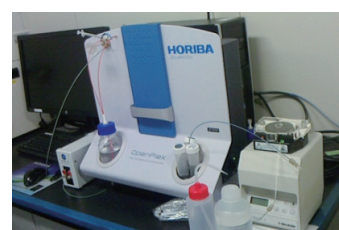
Fig.3 Immunosensor based on surface plasmon resonance (SPR) for multi-targets residual pesticide in agricultural products.
