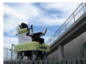
Omnidirectional wheelchair robot being developed at the Center for Symbiotic Human Robotics Research
