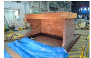
Fig.1: Collapse of the masonry wall specimen with a wooden slab. (Figure)
