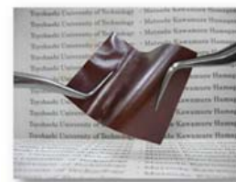
Fig.1: Photograph of the newly developed inorganic-organic composite electrolyte membrane for the advanced fuel cell systems operating at medium temperature without humidification.
