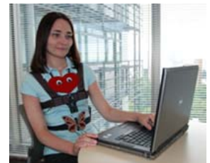
Fig.1. A user communicating through iFeel_IM! (Intelligent System for Feeling Enhancement Powered by Affect-Sensitive Instant Messenger). The devices worn on the body reinforce the communicators' own feelings or simulate the partner's emotions.
