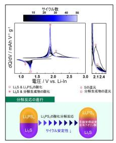
Title: Science of redox reactions in all-solid-state lithium-sulfur batteriesCaption: Redox peak based on differential capacity curve of all-solid-state lithium-sulfur batteries (above)Decomposition of solid electrolytes in cathode composites (below)
