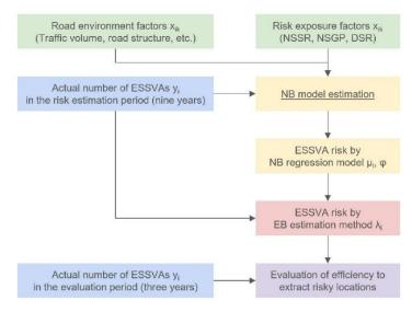
Process for identifying potentail dangerous locations using established statistical model
