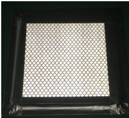
Caption: Surface appearance and structure of RR plate.
