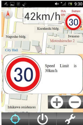
Caption: The mobile application that the research team developed and used for ISA field experiments in 2014 ~ 2015.
