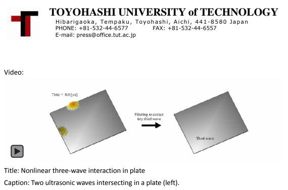
Third ultrasonic wave extracted by filtering (right).
