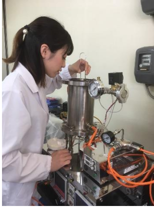
Caption: Setting up a sample in an air-pressure control atmosphere furnace
