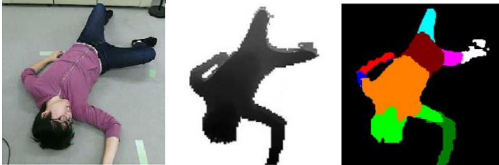
Fig. 1: Example of pose estimation using depth data:
