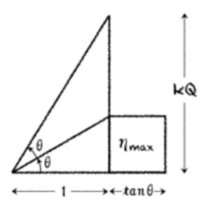
As indicated in the chart, to construct a highly efficient wireless transfer system, it is first necessary to increase kQ. This needs to be considered before providing external reactor elements<sup>\*13.</sup> This is because once energy is lost in the transfer coupler, it cannot be retrieved regardless of how many external elements are added. This is why kQ is an essential design criterion for a wireless transfer.
