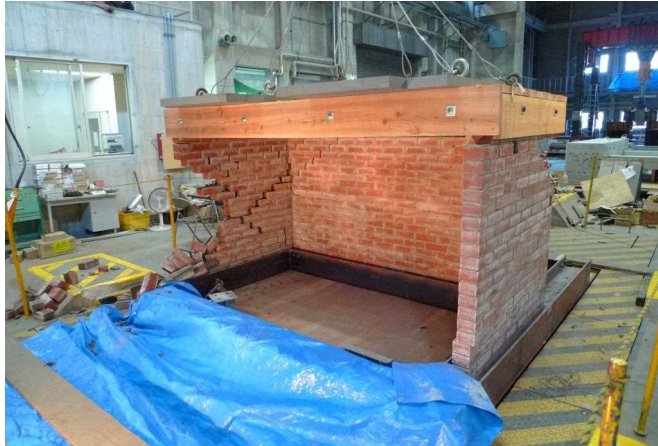
Caption: Collapse of the masonry wall specimen with a wooden slab.
