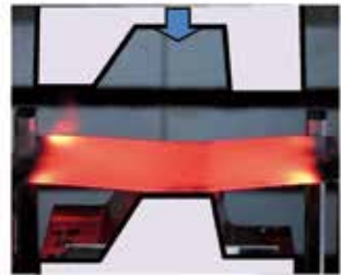
Hot stamping of ultra-high strength steel part
