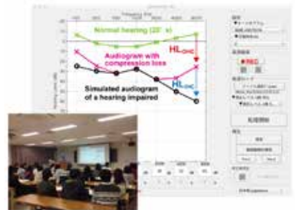
GUI of the hearing impaired simulation system (right) in a practical class for speech therapists (left)
