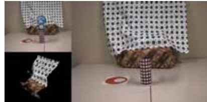
Diminished reality. Left top: input image, left bottom: reconstructed background, right: output image.
