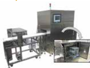
Metallic contaminant detection system using HTS-SQUID. Inset shows the appearance of the electromagnetic shield with SQUID electronics when the front door is open.
