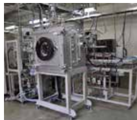
Apparatus for generating high-purity carbon plasma beam
