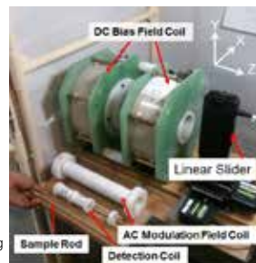
Magnetic Nanoparticle imaging Scanner using HTS-SQUID.
