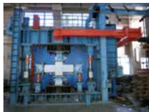
Static loading test of CES beam-column joint
