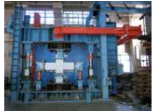
Static loading test of CES beam-column joint
