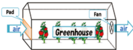
Plant factory equipped with a pad and fan evaporative cooling system
