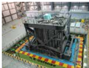
A pile and foundations fracture experiment using a big shaking table
