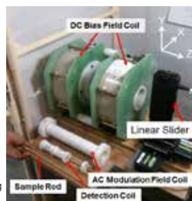
Magnetic Nanoparticle imaging Scanner using HTS-SQUID.
