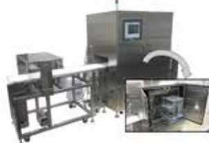
Metallic contaminant detection system using HTS-SQUID. Inset shows the appearance of the electromagnetic shield with SQUID electronics when the front door is open.
