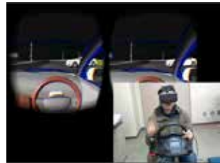
Experiment of back-parking assist system using driving simulator
