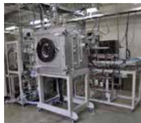
Apparatus for generating high-purity carbon plasma beam
