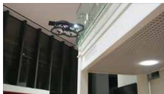
Multicopter for inspection of a wall surface (Fig. 2)
