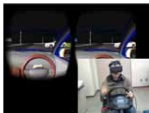
Experiment of back-parking assist system using driving simulator
