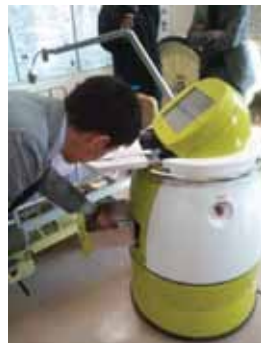
Figure 2. Terapio, a robot supporting medical rounding in a hospital
