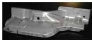
Cold stamping of ultra-high strength steel sheet
