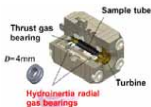
Rotor-bearing system for ultra-high-speed rotating machineries
