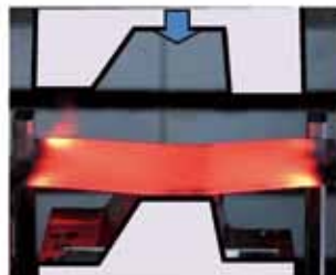
Hot stamping of ultra-high strength steel part
