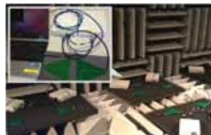
Wireless multi-hop communication testbed using two directional transceivers.
