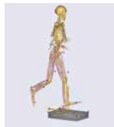
Analysis of landing reaction force using musculo-skeletal model
