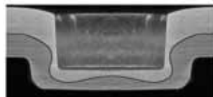
Mechanical clinching of high strength steel and aluminum alloy sheets
