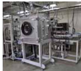
Apparatus for generating high-purity carbon plasma beam
