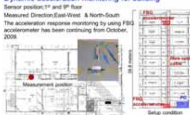
SHM system using FBG accelerometer in Toyohashi Tech.
