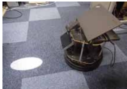
Autonomous robot navigation system using ellipse detection.
