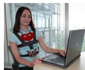
Fig.1. A user communicating through iFeel_IM! (Intelligent System for Feeling Enhancement Powered by Affect-Sensitive Instant Messenger). The devices worn on the body reinforce the communicators' own feelings or simulate the partner's emotions.
